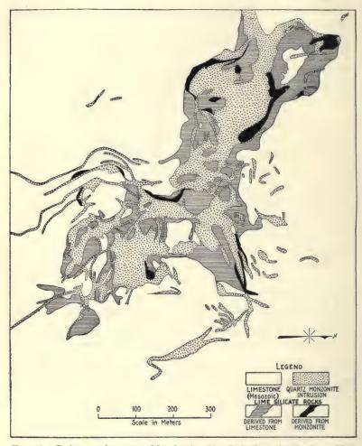
Fig. 53.—Dolores mine area, Matehuala, San Luis Potosi, Mexico. Map showing lime-silicate rocks, derived from alteration of monzonite and of limestone.
